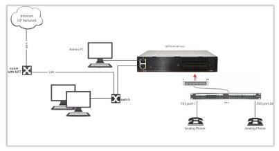
Figure 8: Stand-alone gateway (QXFXS24): Connection overview
