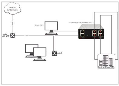
Figure 7: Stand-alone gateway (QXFXO4, QXE1T1 or QXISDN4): Connection overview
