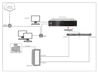
Figure 9: Stand-alone gateway with Legacy PBX (QXFXS24): Connection overview
