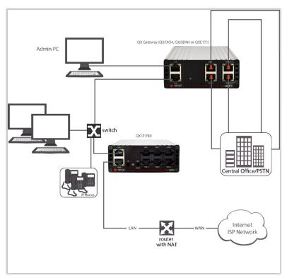
Figure 10: QX gateway (QXFXO4, QXE1T1 or QXISDN4) in shared mode: Connection overview
